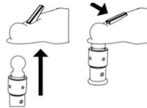
4. Using the Spanner Wrench, turn the Locking Nut counter clockwise until the nut is secured flat against the coupler.
