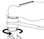
**WARNING!** Failure to tighten the Locking Nut against the coupler may cause the ball to slip out of the coupler.
