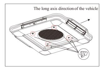
• Fix the plenum assembly on the plenum mounting bracket with four ST4.2×19 pan head screws.
